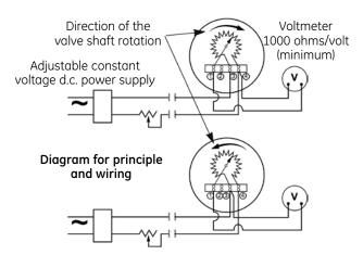
**Zero** is set by orientation of large gear on the rotary shaft from the position of the potentiometer shaft corresponding to the selected zero.
